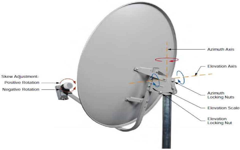
Antenna look-angle adjustments.
